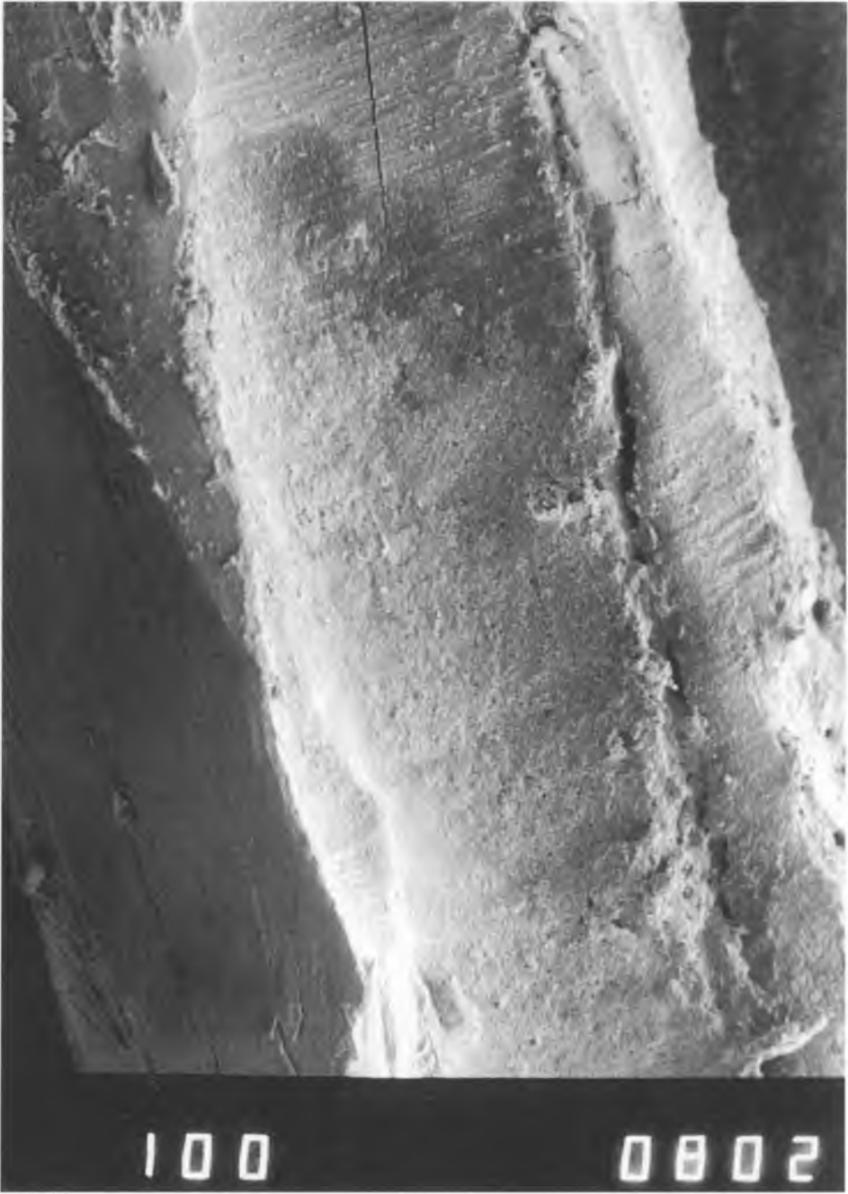
Fig. 4. Tetric after 168 hours – Tetric material (T) applied. Visible marginal adhesion of the material to enamel (S)
