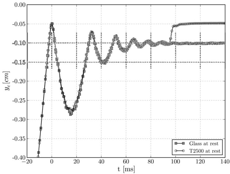
Fig. 3. Variations of the positions of the bubble geometrical center, in respect to the solid/liquid interface, during the bubble bouncing from the glass and Teflon surfaces.
