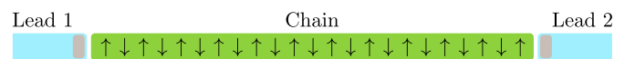
FIG. 15. Schematic representation of system used in the differential conductance G calculation—AFM chain connected to two normal leads. Due to the Coulomb blockade between leads and chains, a barrier region exists in the system (gray area).
