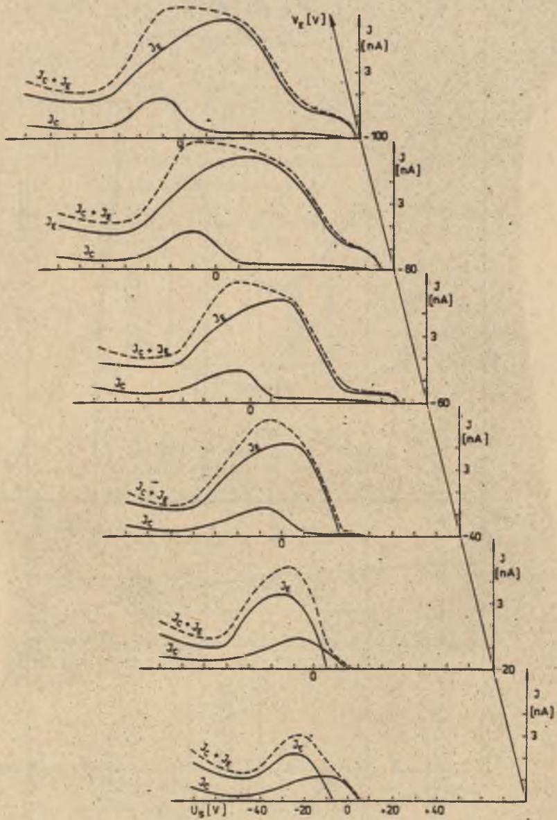
Fig. 3. The dependence current intensity of the collector  $I_C$  and cone electrode  $I_E$  versus the probe voltage  $U_S$  at the various potential  $V_E$ .
