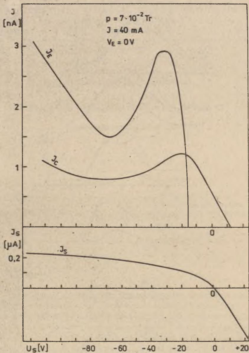
Fig. 2. Typical extraction probe characteristic  $I_s = f(U_s)$  and dependence current intensity of the collector  $I_C$  and cone electrode  $I_E$  versus the probe voltage  $U_s$ .
