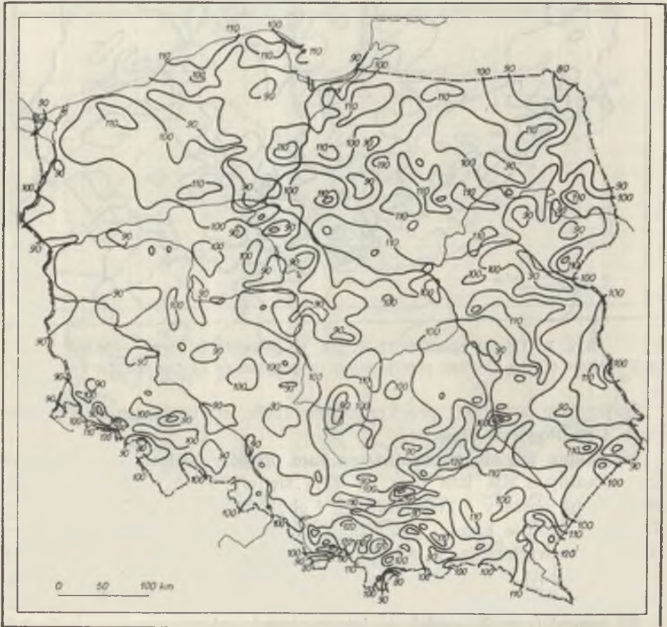
Ryc. 8. Udział opadów 15-letnich w procentach normy — zima Participation of the 15-year precipitation in percentage of the standard — winter
