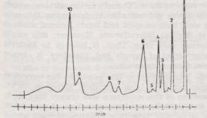
Fig. 6. Chromatogram of fatty acids in beeswax from the GUR Co.; 1 solvent (13% BF; in methanol), 2 palmitic acid, 3 — stearic acid, 4 oleic acid, 5 — oleidic acid, 6 — arachidic + eicosenic acids, 7 — behenic acid, 8 — erucic acid, 9 — lignoceric acid, 10 — nervonic acid
