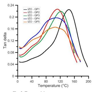
Fig. 3. Tangent delta versus temperature.
