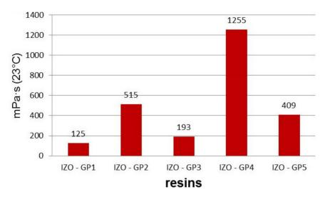
Fig. 1. The viscosity of the resins.
