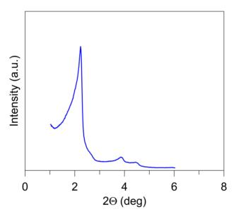
Fig. 5. X-ray diffraction pattern of MCM-41 silica under study.
