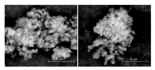
Fig. 6. Representative SEM images of MCM-41 silica material.
