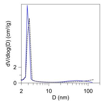
Fig. 4. The pore size distribution for MCM-41 silica calculated by BJH procedure – dash line - adsorption branch, solid line - desorption branch.
