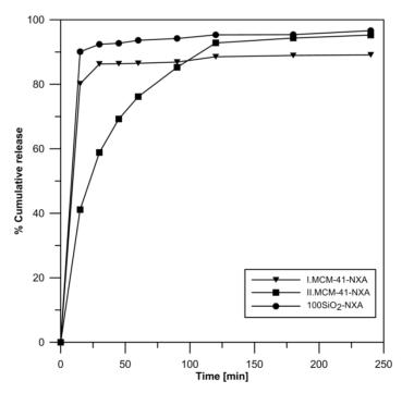
Fig. 7. Naproxen release curves from MCM-41(triangles – sample without outgassed; squares – sample with outgassed) and SiO<sub>2</sub>-100 (circles) silica material.
