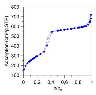
Fig. 3. Nitrogen adsorption (full points)/desorption (open points) isotherms at -196°C of MCM-41 silica.
