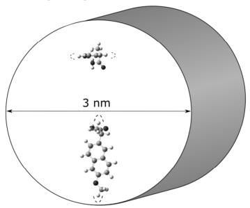
Fig. 9. Schematic comparison of the size (width and length) of Naproxen molecule to the diameter of MCM-41 pore (assumed as 3 nm).
