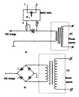
Fig. 4. Use of thyristors as switching devices: (a) half-wave rectifier, (b) full-wave rectifier. Transformator is optional
