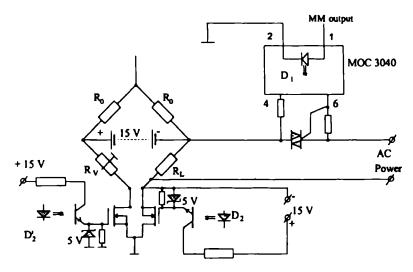
Fig. 3. Details of the switching devices  $K_1$ ,  $K_2$  and  $K_3$  from Fig. 2 Diodes  $D_2$  and  $D'_2$  are connected in series. Two MOSFET transistors and two optically coupled isolators CNY17 were used
