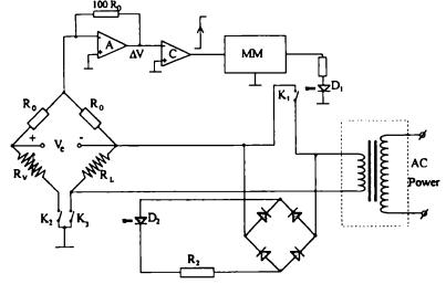
Fig. 2. Economic circuit with single switching device in AC power loop. Transformator is optional
