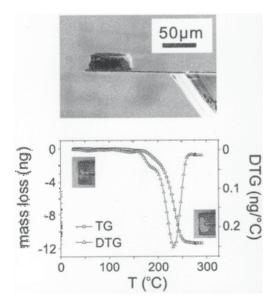
Fig. 10. Scanning electron micrograph of a zeolite single crystal on a micromechanical cantilever. Heating of the sample (TG) resulted in a mass loss of 12 ng. Furthermore the differential mass loss is (DTG) is plotted. © Rüdiger Berger.
