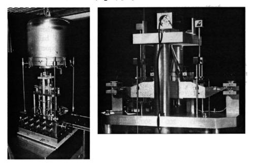
Fig. 9. Flexure-strip balance FB-2, © Bureau International des Poids et Mesures (BIPM), Sèvres, France.
