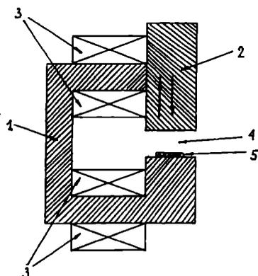
Fig. 1. Block diagram of electromagnet: 1 — magnetic core; 2 — mobile magnetic core; 3 — field coils; 4 — air gap; 5 — sample of seeds
