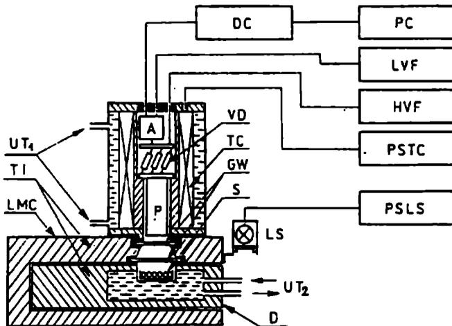
Fig. 2. Block diagram of measuring apparatus [8]: LMC — light-proof measurement chamber, TI — thermal insulator, D — drawer, S — sample, GW — glass windows, P — photomultiplier, VD — voltage divider, A — amplifier, DC — discriminator, PC — pulse counter, LVF — low-voltage feeder, HVF — high-voltage feeder, PSTC — power supply of thermoelectric cooler TC, PSLS — power supply of light source LS, UT<sub>1</sub> and UT<sub>2</sub> — stub pipe for water addition from ultrathermostats
